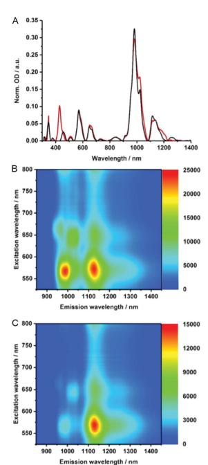
Fig. 3 (A) Normalized absorption spectra of (6,5)-enriched SWCNTs (black), and MINT-por (red) in D<sub>2</sub>O/SDBS (1 wt%, rt), baseline-corrected and normalized to the (7,6)-SWCNT absorption at 1136 nm. 3D nIR fluorescence spectra of (B) (6,5)-enriched SWCNTs and (C) MINT-por in D<sub>2</sub>O/SDBS (1 wt%, rt) with OD of 0.21 at 570 nm.
