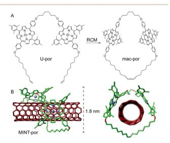
Fig. 1 (A) Chemical structures of U-por and mac-por. (B) Side and front view of the energy-minimized structure (HF-3c) of MINT-por, showing the diameter of the macrocycle. C atoms in green (mac-por) or dark red (SWCNT), N in blue, O in red, Zn in metallic gray. H atoms omitted for clarity.
