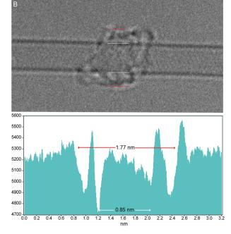
Fig. 2 (A) AFM topographic image of a suspension of MINT-por in TCE and corresponding height profiles along the lines marked in the topographic image. (B) AC-HRTEM image of an individual SWCNT functionalized by a single macrocycle in MINT-por and corresponding profiles (white lines and arrows mark SWNT diameter, red lines and arrows mark mac-por diameter).
