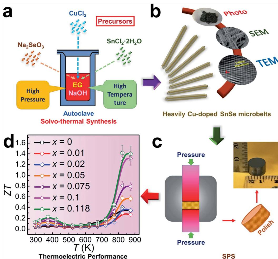
Fig. 1 Illustrations of heavily Cu-doped SnSe ( $\text{Sn}_{1-x}\text{Cu}_x\text{Se}$ ): (a) fabrication process; (b) characterization techniques used; (c) sintering process and (d) obtained  $ZT$  values.
