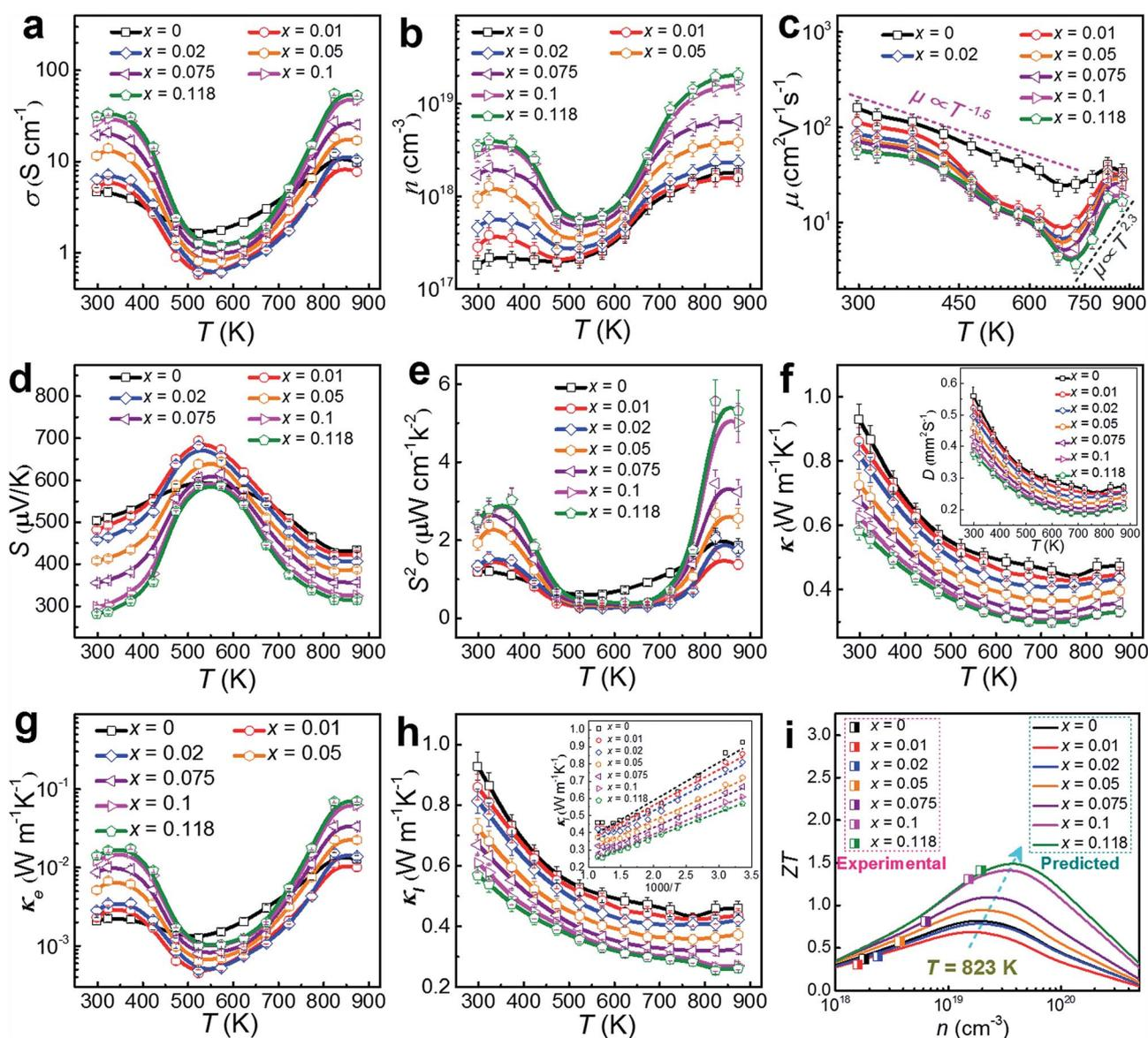
Fig. 6 Plots of measured properties of (a)  $T$ -dependent  $\sigma$ ; (b)  $T$ -dependent  $n$ ; (c)  $T$ -dependent  $\mu$ ; (d)  $T$ -dependent  $S$ ; (e)  $T$ -dependent  $S^2\sigma$ ; (f)  $T$ -dependent  $\kappa$  with inset of  $T$ -dependent  $D$ ; (g)  $T$ -dependent  $\kappa_e$ ; (h)  $T$ -dependent  $\kappa_l$  with inset of  $1000/T$ -dependent  $\kappa_l$  and (i) comparison of experimental ZTs with predicted plots for our Cu-doped SnSe pellets.
