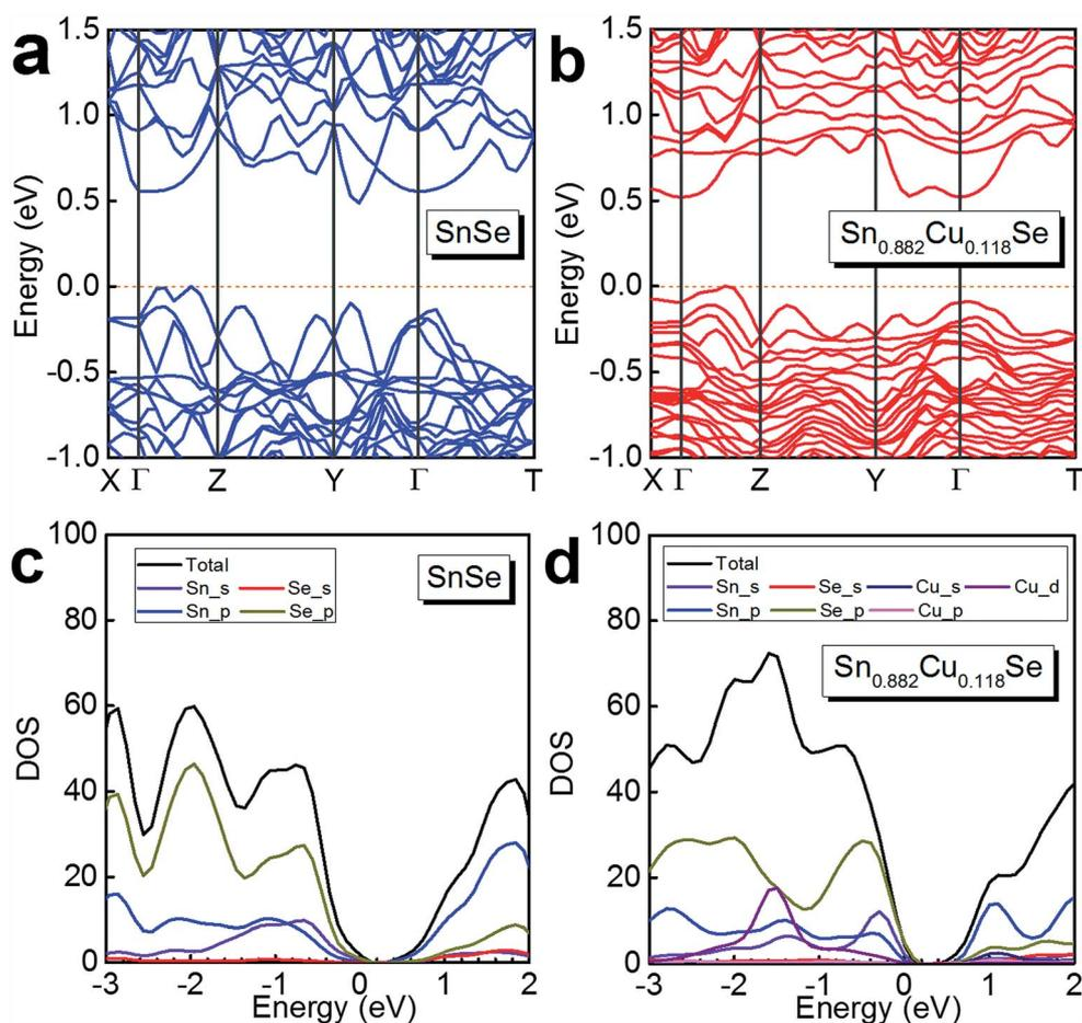
Fig. 7 Calculated band structure of (a) SnSe and (b)  $\text{Sn}_{0.882}\text{Cu}_{0.118}\text{Se}$ , and the calculated density of states (DOS) of (c) SnSe and (d)  $\text{Sn}_{0.882}\text{Cu}_{0.118}\text{Se}$ .
