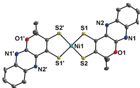
Fig. 10 X-ray crystal structure of a  $\text{Ni}^{\text{III}}$ (bis-dithiolene) complex with a quinoxaline-pyran-fused dithiolene dianion ligand ( $\text{qpdt}^{2-}$ ) ( $[\text{Ni}^{\text{III}}(\text{qpdt})_2]^-$ ) at 50% probability. Hydrogen atoms are omitted for clarity. Reprinted with permission from ref. 138. Copyright 2018, American Chemical Society.
