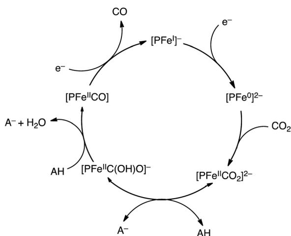
Scheme 3 Catalytic cycle for two-electron reduction of  $\text{CO}_2$  to  $\text{CO}$  with an iron porphyrin ( $[\text{PFe}]^{2-}$ ).<sup>84</sup>
