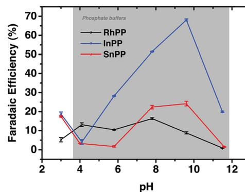
Fig. 9 Faradaic efficiencies for the electrocatalytic reduction of CO<sub>2</sub> to HCOOH or HCOO<sup>-</sup> with RhPP, InPP and SnPP, determined at *t* = 10 min, at *E* = -1.5 V vs. RHE as function of pH. Reprinted with permission from ref. 126. Copyright 2017, Elsevier.
