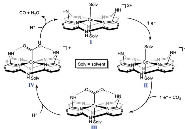
Scheme 5 Catalytic cycle of two-electron reduction of CO<sub>2</sub> to CO with a nonheme cobalt complex with a macrocyclic aminopyridine (**I**). Reprinted with permission from ref. 96. Copyright 2016, American Chemical Society.
