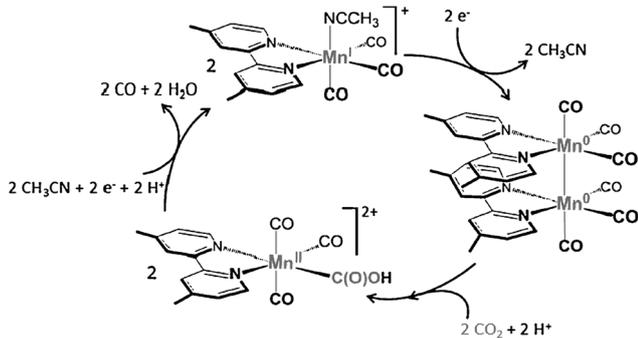
Scheme 6 The catalytic cycle for two-electron reduction of CO<sub>2</sub> to CO with [Mn(bpy)(CO)<sub>3</sub>]<sup>+</sup>. Reprinted with permission from ref. 113. Copyright 2014, WILEY-VCH Verlag GmbH.
