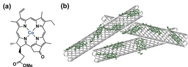
Fig. 3 (a) Structure of  $\text{Co}^{\text{II}}(\text{Ch})$  and (b) schematic image of  $\text{Co}^{\text{II}}(\text{Ch})$  on MWCNTs. Reprinted with permission from ref. 91. Copyright 2015, Royal Society of Chemistry.
