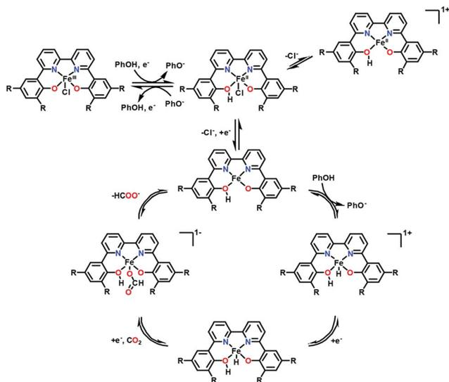
**Scheme 8** Catalytic cycle for two-electron reduction of CO<sub>2</sub> to CO with a nonheme iron(III) chloride bearing a 6,6'-di(3,5-di-*tert*-butyl-2-hydroxybenzene)-2,2'-bipyridine ligand (Fe<sup>(*tbu*)dhbpy</sup>)Cl) via protonation by phenol. Reprinted with permission from ref. 127. Copyright 2018, American Chemical Society.
