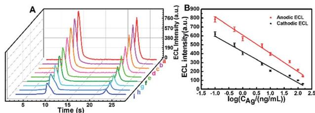
Fig. 4 (A) ECL-time profiles of the electrode at different concentrations of Ag (a–i: 0, 0.1, 0.5, 1, 5, 10, 50.0, 100.0 and 150.0 ng mL $^{-1}$ ). (B) Relationship between ECL $_{\text{anode}}$  vs. log  $C_{\text{Ag}}$  (red line) and ECL $_{\text{cathodic}}$  vs. log  $C_{\text{Ag}}$  (black line).
