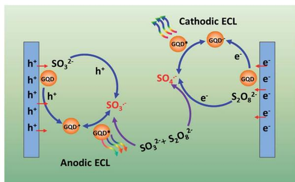
Scheme 1 Schematic illustration of the ECL mechanism of GQDs.
