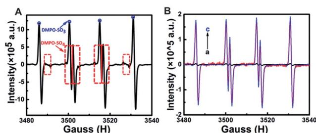
Fig. 3 (A) EPR spectrum of  $\text{K}_2\text{S}_2\text{O}_8$ – $\text{Na}_2\text{SO}_3$ –DMPO. (B) (a) EPR spectrum of DMPO– $0.1$  M  $\text{Na}_2\text{SO}_3$  in a cyclic potential scan from  $0$  to  $1.5$  V. (b) EPR spectrum of DMPO– $0.1$  M  $\text{Na}_2\text{SO}_3$ – $0.01$  M  $\text{K}_2\text{S}_2\text{O}_8$ . (c) EPR spectrum of DMPO– $0.1$  M  $\text{Na}_2\text{SO}_3$ – $0.01$  M  $\text{K}_2\text{S}_2\text{O}_8$  in a cyclic potential scan from  $0$  to  $1.5$  V.
