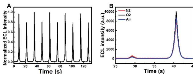
Fig. 2 (A) Continuous ECL responses of the GQDs–K<sub>2</sub>S<sub>2</sub>O<sub>8</sub>–Na<sub>2</sub>SO<sub>3</sub> system during a continuous potential scan between –1.2 and 1.5 V at a scan rate of 0.2 V s<sup>-1</sup> (B) ECL-time profiles of the GQDs–K<sub>2</sub>S<sub>2</sub>O<sub>8</sub>–Na<sub>2</sub>SO<sub>3</sub> system in air-saturated (blue curve), nitrogen-saturated (red curve) and oxygen-saturated (black curve) 0.1 M PBS (pH 7.4) (scan potential: –1.2 to 1.0 V).
