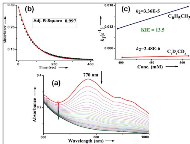
Fig. 8 (a) UV-vis change during the bromination of toluene, (b) inset 770 nm decay plot of **2** during the bromination of toluene, (c) kinetic isotope effect study during the bromination reaction (kinetic studies were carried out under a  $N_2$  atmosphere at 25 °C).
