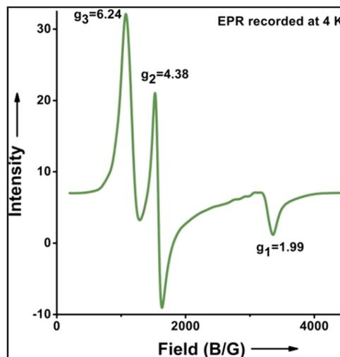
Fig. 7 EPR spectrum showing one electron oxidation of **6** using 0.5 of *m*CPBA (temperature 4 K, X-band frequency 9.376 GHz, modulation amplitude 4G, modulation frequency 100 kHz, and attenuation 22 dB).
