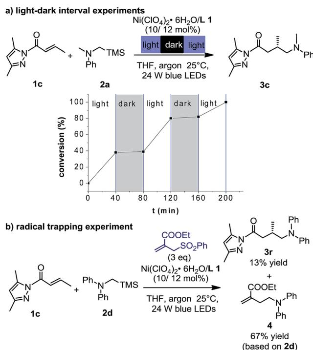
Fig. 3 Mechanistic investigation. (a) Intervals of irradiation and dark periods for the nickel-catalyzed reaction **1c** + **2a** → **3c**. (b) Radical trapping experiment in the nickel-catalyzed reaction **1c** + **2d** → **3r**.
