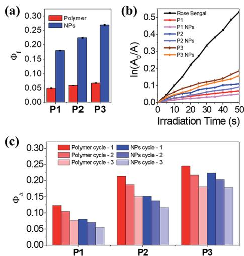
Fig. 4 (a)  $\Phi_f$  of P1–P3 and the P1–P3 NPs in HEPES buffer (10 mM, pH 7.0) at 25 °C. (b) Plot of  $\ln(A_0/A)$  as a function of time of visible light irradiation on the various photosensitizers, where  $A_0$  and  $A$  are absorption intensity at 400 nm at the beginning and at irradiation time  $t$ , respectively. (c)  $\Phi_\Delta$  of P1–P3 and the P1–P3 NPs in HEPES buffer/D<sub>2</sub>O (V/V = 1 : 9).
