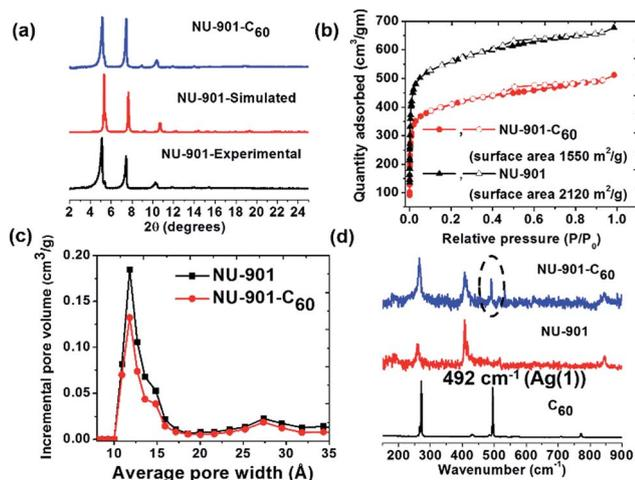
**Fig. 2** (a) PXRD pattern of simulated NU-901, experimental NU-901, and experimental NU-901- $C_{60}$ , (b)  $N_2$  adsorption-desorption isotherms (77 K) (NU-901 and NU-901- $C_{60}$ ), (c) density functional theory (DFT) pore size distribution (NU-901- $C_{60}$  and NU-901) and, (d) Raman spectra (NU-901, NU-901- $C_{60}$  and  $C_{60}$ ).
