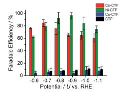
Fig. 3 Effect of potential on the faradic efficiency values during the  $CO_2RR$  to generate CO using Co-CTF (red), Ni-CTF (green), Cu-CTF (blue) and CTF (black) in a KHCO $_3$  electrolyte (saturated with  $CO_2$ ) at pH 6.8. The error bar represents the standard deviation from three experimental trial.
