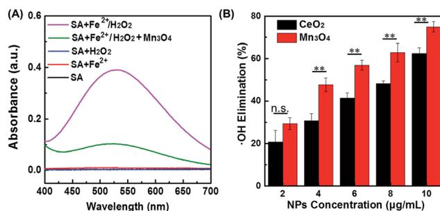
Fig. 4 (A) Absorption spectra of SA after reaction with  $\text{Fe}^{2+}/\text{H}_2\text{O}_2$ , in the absence and presence of  $\text{Mn}_3\text{O}_4$  NPs. SA alone, and SA reacted with  $\text{Fe}^{2+}$  or  $\text{H}_2\text{O}_2$  were used as control. (B) Dependence between the elimination of  $\cdot\text{OH}$  and concentration of  $\text{Mn}_3\text{O}_4$  NPs and  $\text{CeO}_2$  NPs (mean  $\pm$  S.D., \*\* $p < 0.05$ ; n.s., not significant).
