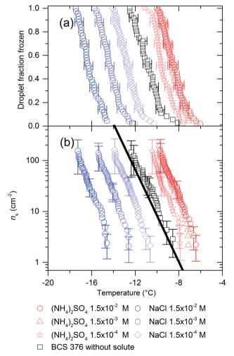
Fig. 2 (a) Fraction frozen curves and (b)  $n_{\rm s}(T)$  values for 0.1 wt% of BCS 376 microcline suspended in various concentrations of (NH<sub>4</sub>)<sub>2</sub>SO<sub>4</sub> and NaCl. The black line is the paramaterisation for the ice nucleation activity of BCS376 microcline from Atkinson  $et~al.^{28}$  It can be seen that reduced concentrations of solutes lead to smaller impacts on freezing temperatures.
