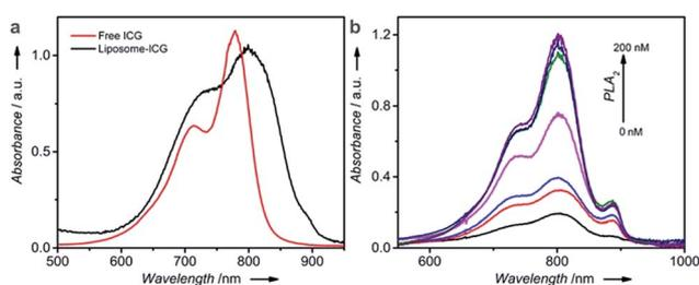
Fig. 1 (a) UV-vis spectra of free ICG and liposome-ICG. (b) UV-vis spectra of the supernatant collected after incubating liposome-ICG with different concentrations of PLA<sub>2</sub> for 2 h. Bottom to top: 0, 5, 10, 20, 50, 100, and 200 nM.
