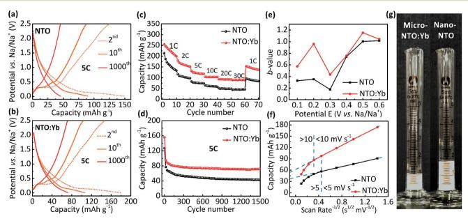
Fig. 2 The 2<sup>nd</sup>, 10<sup>th</sup>, and 1000<sup>th</sup> charge/discharge curves of (a) NTO and (b) NTO:Yb. (c) The rate and (d) cycle performance of NTO and NTO:Yb in a half cell. (e) b-values for NTO and NTO:Yb as a function of potential for anodic sweeps (Na<sup>+</sup> insertion). (f) Capacity v-rsus v-1/2 allows for the separation of diffusion-controlled capacity from capacitive-controlled capacity. (g) The comparison of tap densities of nano-NTO and micro-NTO:Yb.
