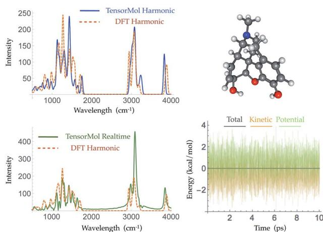
Fig. 7 The geometry of morphine as optimized by TensorMol-0.1 (upper right panel) and its harmonic IR spectra simulated using  $\omega\text{B97X-D/6-311G}^{**}$  (dashed orange line) and the TensorMol force field (solid blue line) (upper left panel). The lower panels show the real-time IR spectra obtained using TensorMol (solid green line), and the DFT results (dashed orange line) (left), and the conservation of energy maintained by the smoothness of the energy (right).
