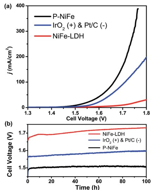
Fig. 7 (a) LSV curves of P-NiFe (black) and NiFe-LDH (red) as HER and OER bifunctional catalysts in 1.0 M KOH solution for overall water splitting.  $\text{IrO}_2$  and Pt/C as OER and HER benchmarks were measured for comparison (blue). (b) Current density traces of CCE at  $10 \text{ mA cm}^{-2}$  for overall water splitting in 1.0 M KOH for P-NiFe (black), NiFe-LDH (red), and commercial benchmarks of  $\text{IrO}_2$  and 20% Pt/C (blue).
