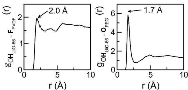
Fig. 6 Radial distribution functions for the most preferential MOF/polymer interactions for the UiO-66/PVDF (left) and UiO-66/PEG (right) interfaces.
