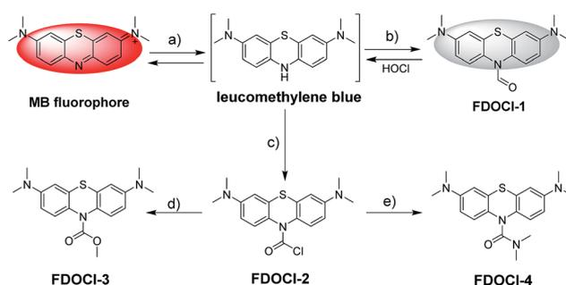
**Scheme 1** Structures and detecting mechanisms of prepared probes for HOCl. The reagents are: (a) Na<sub>2</sub>S<sub>2</sub>O<sub>4</sub> and Na<sub>2</sub>CO<sub>3</sub>; (b) the Vilsmeier–Haack reagent; (c) bis(trichloromethyl) carbonate; (d) 4-dimethylaminopyridine, Na<sub>2</sub>CO<sub>3</sub> and MeOH; and (e) Na<sub>2</sub>CO<sub>3</sub> and dimethylamine.
