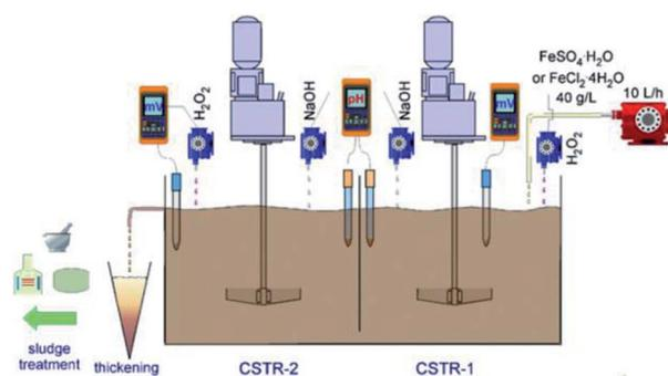
Fig. 3 Scheme of the laboratory iron oxy-hydroxides' production.<sup>52</sup>
