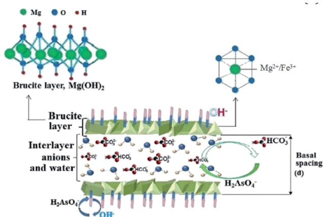
Fig. 9 Schematic mechanism of As(V) adsorption on Mg–Fe– $\text{CO}_3^{2-}$ -LDHs.<sup>197</sup>
