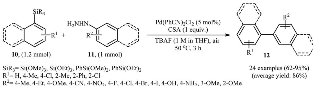
Scheme 6 Denitrogenative Hiyama cross-coupling of aryl silanes **10** with arylhydrazines **11** developed by Zhang.
