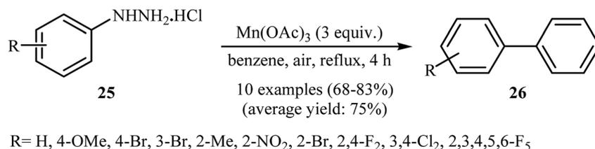
Scheme 14 Mn(OAc)<sub>3</sub>-mediated oxidative coupling of benzene with arylhydrazines 25.
