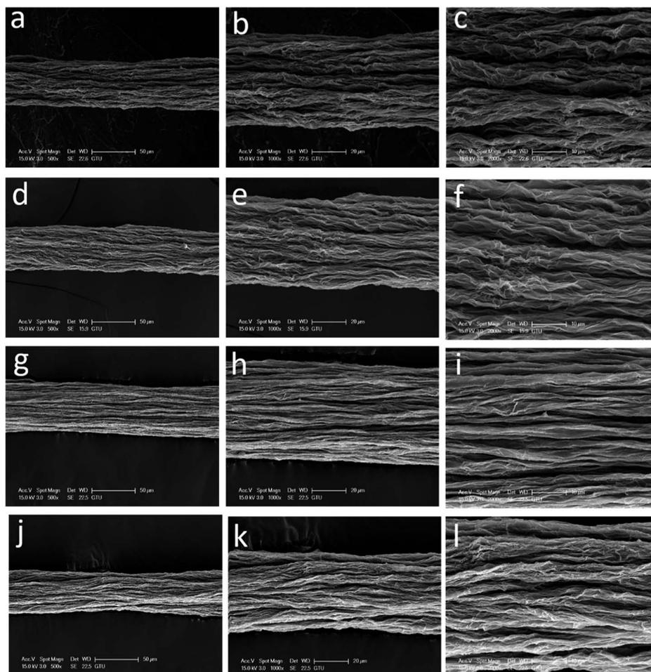
Fig. 6 SEM images of GFs obtained by reducing the dried GOFs obtained by using isopropanol coagulation baths at different temperatures under different magnifications (500 $\times$ , 1000 $\times$  and 2000 $\times$ ): (a–c) GF@35 $^{\circ}$ -IPA; (d–f) GF@25 $^{\circ}$ -IPA; (g–i) GF@15 $^{\circ}$ -IPA; (j–l) GF@5 $^{\circ}$ -IPA.
