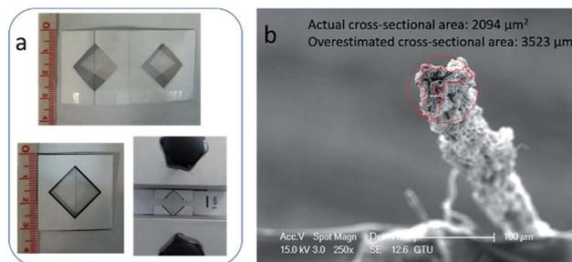
**Fig. 3** (a) The paper frames used during the tensile tests; (b) SEM image of GOF@25°-IPA sample after the rupture during the tensile test to calculate their cross-section.
