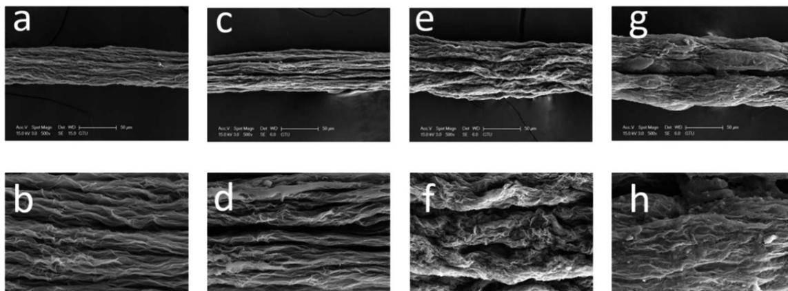
**Fig. 5** SEM images of GFs obtained by reducing dried GOF@25°-IPA by different chemical agents: 500 $\times$  and 2000 $\times$  magnification (a and b) reduced graphene filament by HI/AAC, (c and d) reduced graphene filament by HI, (e and f) reduced graphene filament by AsAc, (g and h) reduced graphene filament by Hdz.
