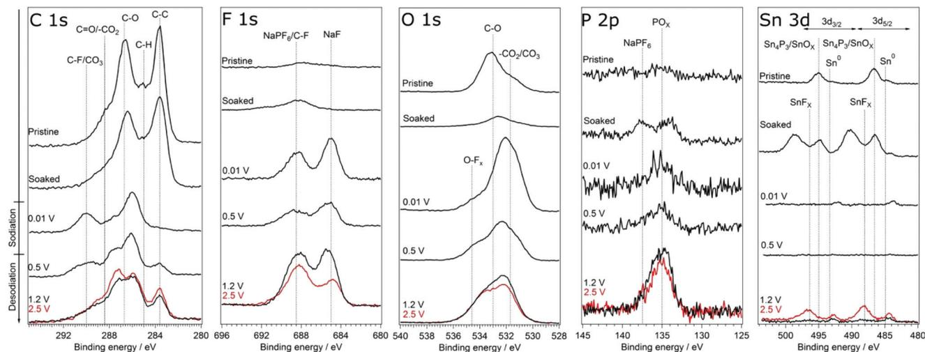
Fig. 6 HAXPES spectra of  $\text{Sn}_4\text{P}_3$  electrodes from cells with the  $\text{NaPF}_6$  based electrolyte. The spectra were measured using photon energy of 2005 eV. The samples charged to 2.5 V is shown in red.
