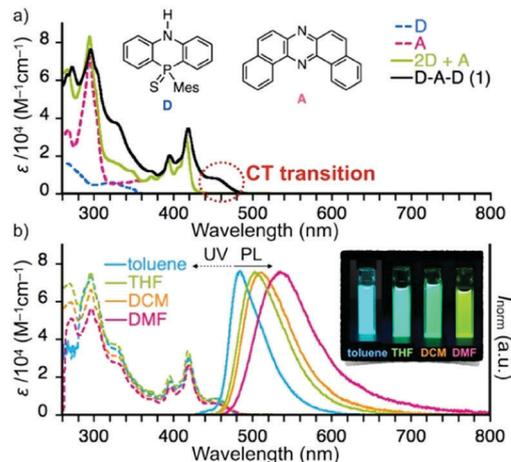
Fig. 2 (a) UV spectra of DCM solutions ( $c \times 10^{-5}$  M) of D, A, 2D + A, and D–A–D (**1**); (b) UV-vis and steady-state PL spectra of the solutions ( $c \times 10^{-5}$  M) prepared with different solvents. The inset photos were taken under irradiation with UV light ( $\lambda$  365 nm).
