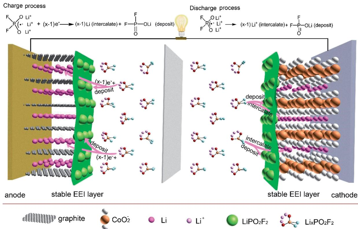
Fig. 6 The schematic of the forming process of SEI on the anode and cathode surfaces in the  $\text{LiCoO}_2/\text{graphite}$  18650 full battery with electrolyte containing  $\text{LiPO}_2\text{F}_2$ , and the reaction on the anode and cathode surfaces during cycle process.
