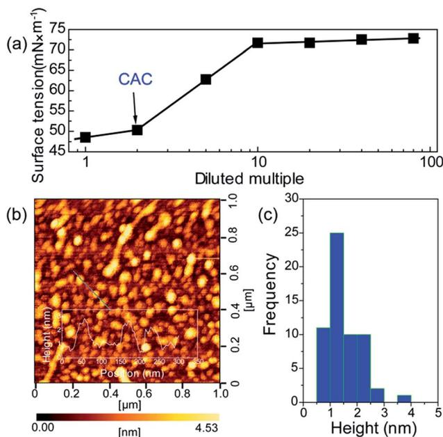
Fig. 4 (a) Surface tension of the mixed solution of DETA and CA at the concentration of 10 mg mL<sup>-1</sup> with diluted multiple at 25 °C micelle formation. (b) AFM topography image of CA–DETA mixed systems and sectional height profile along the line shows inset. (c) Height distribution estimated from (b).
