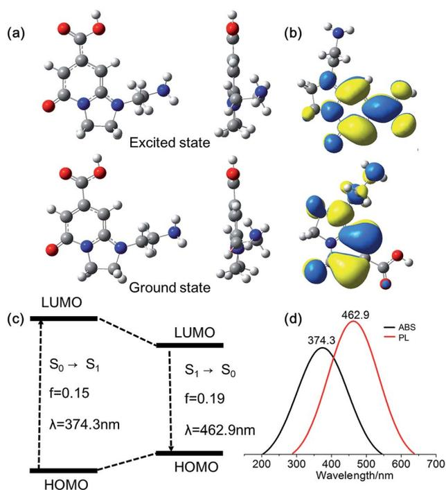
Fig. 6 (a) Optimized geometry of AEOIP molecule in solution. (b and c) The electronic transitions between the ground ( $S_0$ ) and excited ( $S_1$ ) states as reflected by wave functions of frontier orbitals (transitions between HOMO and LUMO) in the single AEOIP molecule in aqueous solution. (d) Calculated absorption and fluorescence emission spectra from Gaussian calculations.
