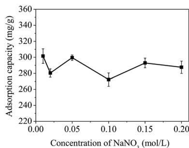
Fig. 10 Effect of ionic strength on the removal of mercury(II). Condition:  $T = 300$  K,  $C_0 = 20$  mg L<sup>-1</sup>, RSL = 0.05 g L<sup>-1</sup>, pH = 7.0 ± 0.1.
