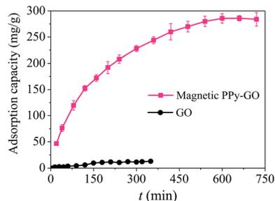
Fig. 11 Effect of time on the removal of Hg(II) with GO and magnetic PPy-GO. Conditions:  $T = 300$  K,  $C_0 = 20$  mg L<sup>-1</sup>, RSL = 0.05 g L<sup>-1</sup> and pH = 7.0 ± 0.1 for magnetic PPy-GO;  $T = 298$  K, RSL = 0.5 g L<sup>-1</sup>,  $C_0 = 100$  mg L<sup>-1</sup> and pH = 6.0 for GO.<sup>32</sup>
