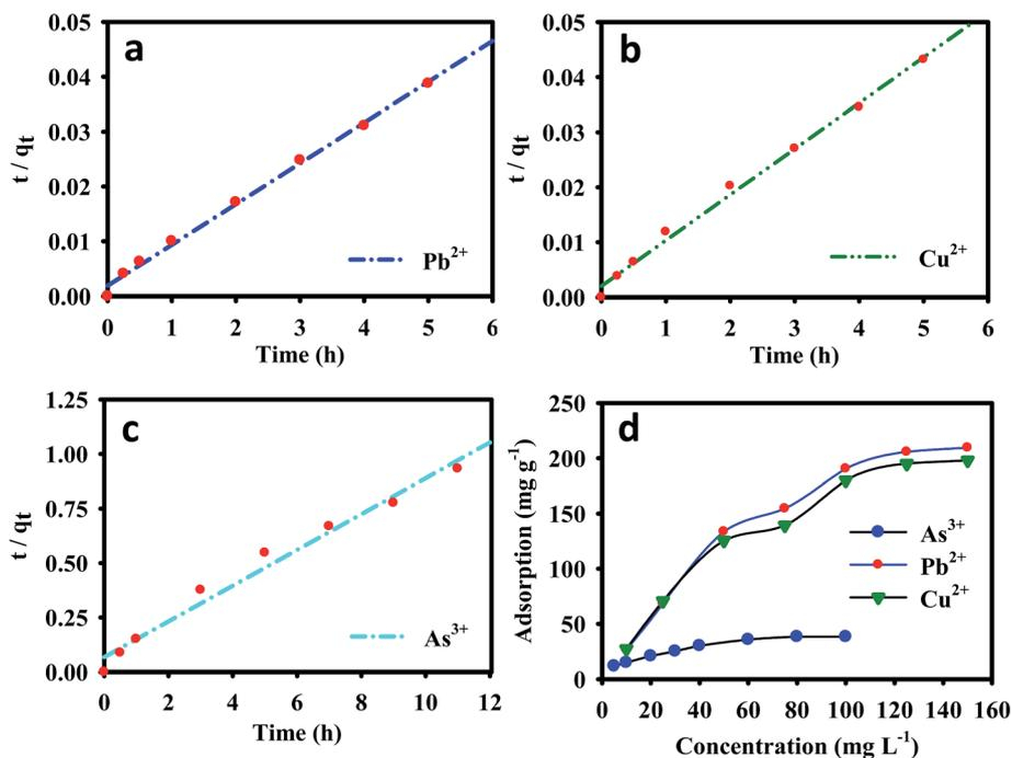
Fig. 3 Pseudo-second-order curve-fitting graphs of (a)  $\text{Pb}^{2+}$ , (b)  $\text{Cu}^{2+}$ , and (c)  $\text{As}^{3+}$  at 298.15 K. (d) Adsorption profiles of  $\text{Pb}^{2+}$ ,  $\text{Cu}^{2+}$ , and  $\text{As}^{3+}$  on EDTA-MCS/GO nanocomposite at different metal ion concentrations.
