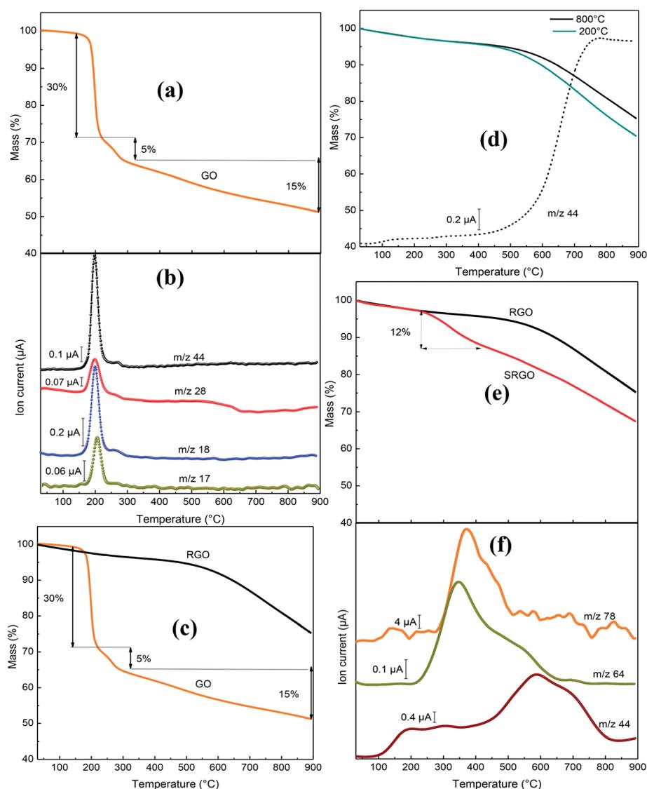
**Fig. 8** (a) Mass variation for GO, (b) MS profile for GO, (c) mass variation for GO and RGO, (d) mass variation for GO following heat treatment at 200 and 800 °C, MS profile (– –) for GO following heat treatment at 800 °C, (e) mass variation for RGO and SRGO and (f) MS profiles for SRGO.
