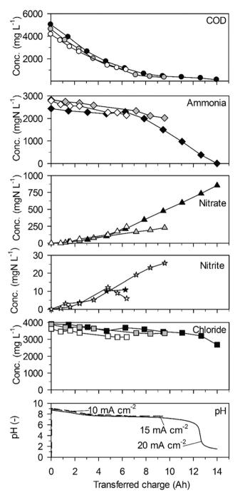
Fig. 1 Galvanostatic electrolysis of high-concentration urine on BDD. Full symbols: 20 mA cm $^{-2}$  (25.2 °C), grey symbols: 15 mA cm $^{-2}$  (25.1 °C) and empty symbols 10 mA cm<sup>-2</sup> (25.0 °C). Electrode gap: 9 mm.
