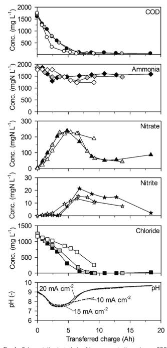
Fig. 4 Galvanostatic electrolysis of low-concentration urine on BDD. Full symbols: 20 mA cm $^{-2}$  (16.5 °C), grey symbols: 15 mA cm $^{-2}$  (16.6 °C) and empty symbols 10 mA cm<sup>-2</sup> (16.2 °C). Electrode gap: 9 mm.
