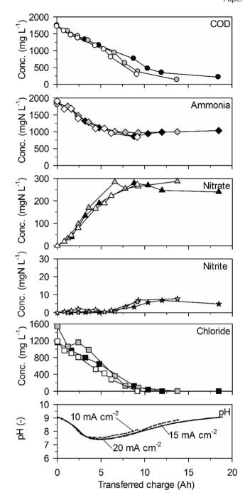
Fig. 5 Galvanostatic electrolysis of low-concentration urine on TDIROF. Full symbols: 20 mA cm $^{-2}$  (16.4 °C), grey symbols: 15 mA cm $^{-2}$ (16.4 °C) and empty symbols 10 mA cm<sup>-2</sup> (16.6 °C). Electrode gap: 10
