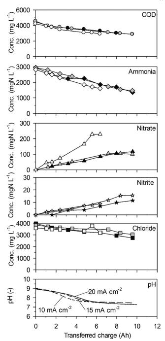
Fig. 2 Galvanostatic electrolysis of high-concentration urine on TDIROF. Full symbols: 20 mA cm $^{-2}$  (25.1  $^{\circ}$ C), grey symbols: 15 mA cm $^{-2}$ (25.0 °C) and empty symbols 10 mA cm $^{-2}$  (25.0 °C). Electrode gap: 10
