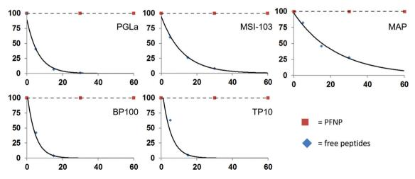
Fig. 6 Degradation of the free peptides in the presence of trypsin occurs rapidly within 30 min while the peptide bound to the gold surface (PFNP) are completely stable during this time.
