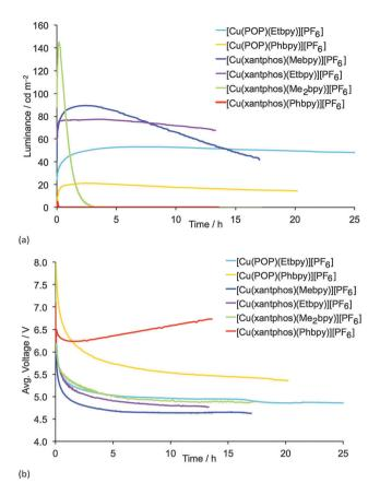
Fig. 10 Luminance (a) and average voltage (b) for ITO/PEDOT: PSS/ [Cu(P^P)(N^N)][PF<sub>6</sub>]: [Emim][PF<sub>6</sub>] 4:1 molar ratio/Al LECs measured using a pulsed current driving (average current density 50 A  $\mathrm{m}^{-2}$ , 1 kHz, 50% duty cycle, block wave). [Emim][PF<sub>6</sub>] = 1-ethyl-3-methylimidazolium hexafluoridophosphate.
