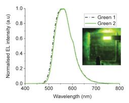
Fig. 3 Electroluminescence (EL) spectra of **Green 1** and **Green 2**. Inset shows a working green OLED.
