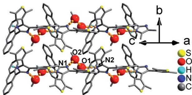
Fig. 2 Supramolecular chain structure in 2. The red balls are the O atoms from the CH<sub>3</sub>OH molecules.
