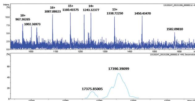
**Fig. 5** ESI-MS of His3 Mn<sup>III</sup>Mb after reacting with 20 equiv. KHSO<sub>5</sub> for 3 min.
