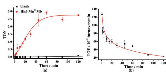
**Fig. 6** Time course plots of (a) turnover number (TON) with or without His3 Mn<sup>III</sup>Mb, and (b) turnover frequency (TOF) of styrene epoxidation catalyzed by His3 Mn<sup>III</sup>Mb. TON and TOF were calculated based on the amount of styrene. The initial TOF was calculated at 1 min.
