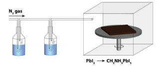
Fig. 1 Schematic of the apparatus used to control the RH inside an atmospheric bag containing a spin coater. Pbl<sub>2</sub> films are converted into CH<sub>3</sub>NH<sub>3</sub>Pbl<sub>3</sub> by immersion in a solution of CH<sub>3</sub>NH<sub>3</sub>I, spin dried at 3000 rpm for 30 s, and allowed to dry for a further 10 min.
