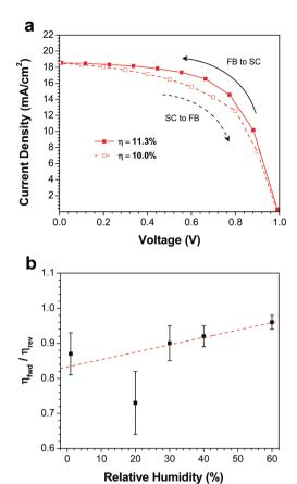
Fig. 5 (a) J-V curves measured at  $0.1 \, \mathrm{V \, s^{-1}}$  for the best device prepared at 40% RH. (b) Ratio of PCEs determined from forward (SC-FB) and reverse (SC-FB) scans as a function of RH. The linear fit is a guide to the eye.
