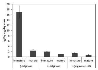
Fig. 3 Effect of 24 hour enzymatic digestion of Macrocystis blade as a function of life cycle. Other conditions as described in the text. Error bars represent ±1 SD from triplicate measurements.
