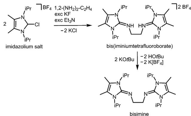
Scheme 15 Synthesis of the bisimine compound 1,2-( $L^{iPr_2Me_2}N$ )<sub>2</sub>-C<sub>2</sub>H<sub>4</sub> ( $L^{iPr_2Me_2} = 1,3$ -diisopropyl-4,5-dimethyl-imidazolin-2-ylidene) from an imidazolium salt precursor.
