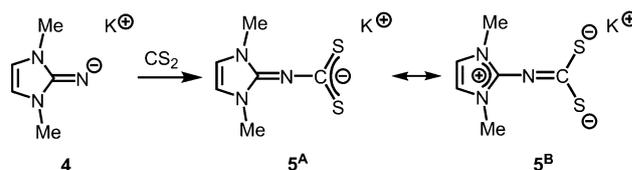
**Scheme 2** Conversion of potassium imide **4** with carbon disulfide to the thiocarbimate **5** (represented by resonance structures **5<sup>A</sup>** and **5<sup>B</sup>**).
