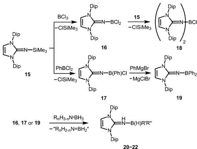
Scheme 6 Conversion of the imino trimethylsilane **15** to the imino boron dichlorides **16–18** and the imino diphenylborane **19**. Formation of the imine–borane adducts via abstraction of dihydrogen from amine–borane adducts.
