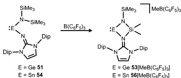
**Scheme 13** Synthesis of four-membered metallyliumylidenes **53<sup>+</sup>** and **56<sup>+</sup>** by methyl-abstraction from the amino(imino)metallylenes **51** and **54**.
