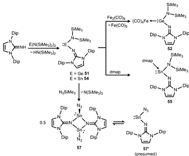
**Scheme 12** Preparation of amino(imino)metallylenes **51** and **54** and the iron carbonyl **52**, as well as the dmap adduct **55** (dmap = 4-dimethylamino-pyridine). Conversion of **54** to dimeric stannylene azide **57**.
