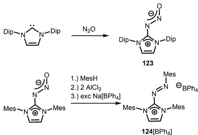
Scheme 28 Synthesis of representative examples for the compound classes: diazotates (**123**) and azoimidazolium salts (**124**[BPh<sub>4</sub>]).
