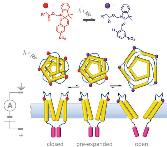
Fig. 14 Semi-synthetic light-gated ion channel prepared from a chemically modified mechanosensitive channel protein.<sup>34</sup>
