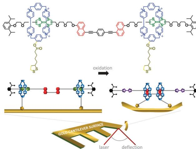
Fig. 6 Cantilever actuation driven by redox switching of surface-bound rotaxane shuttles.<sup>13</sup>
