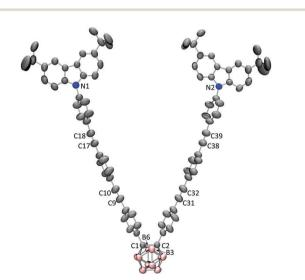
Fig. 1 Crystal structure of **D-3**. Selected bond lengths (Å): C1–C2 1.718(3), C9-C10 1.187(3), C17-C18 1.198(3), C31-C32 1.187(3), C38-C39 1.198(3), C1-N1 19.376, C2-N2 19.376. Hydrogen atoms have been omitted for clarity.
