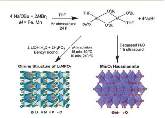
Fig. 1 Reaction schematic for the synthesis of LiMPO<sub>4</sub> (M = Fe or Mn) and Mn<sub>3</sub>O<sub>4</sub> using metal alkoxide precursors.
