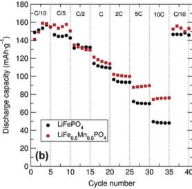
**Fig. 4** (a) Cycling performance and capacity fading (inset) of C/LiFePO<sub>4</sub> prepared from [Fe(O<sup>t</sup>Bu)<sub>2</sub>(THF)]<sub>2</sub> alkoxide precursor (mixed with C black and PTFE in 60:30:10 weight%) between 2.2 and 4.0 V at C/20 rate. (b) Rate performance of C/LiFePO<sub>4</sub> and C/LiFe<sub>0.5</sub>Mn<sub>0.5</sub>PO<sub>4</sub> (mixed with C black and PTFE in 60:30:10) at different charge–discharge C rates.
