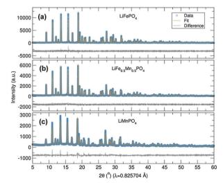
Fig. 2 Rietveld analysis of XRD data of (a) LiFePO<sub>4</sub>, (b) LiFe<sub>0.5</sub>Mn<sub>0.5</sub>PO<sub>4</sub> and (c) LiMnPO<sub>4</sub> nanostructures prepared from [Fe(O<sup>t</sup>Bu)<sub>2</sub>(THF)]<sub>2</sub>, "[Fe<sub>0.5</sub>Mn<sub>0.5</sub>-(O<sup>t</sup>Bu)<sub>2</sub>(THF)]<sub>2</sub>" and "[Mn(O<sup>t</sup>Bu)<sub>2</sub>(THF)]<sub>2</sub>" alkoxides, respectively
