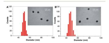
Fig. 4 Size distribution and TEM images (inset) of TAT-TPDC NPs (A) and TAT-PPDC NPs (B).
