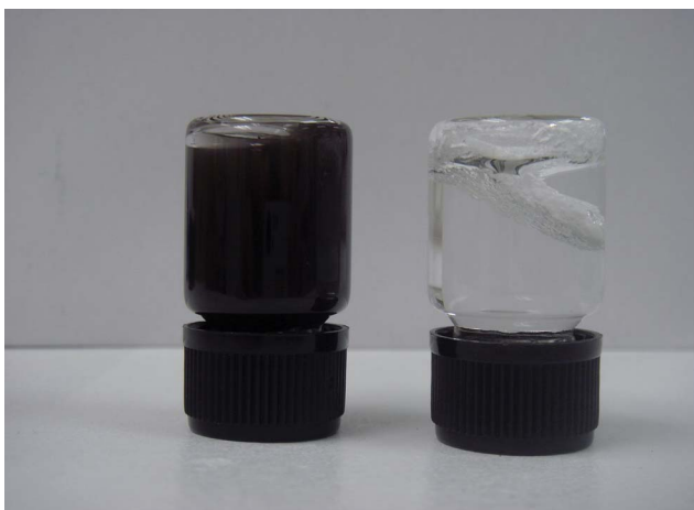
Fig. 1 Photographs of vials containing the pristine BNNTs (right-hand side) and the functionalized BNNTs (left-hand side) in water after standing overnight.
