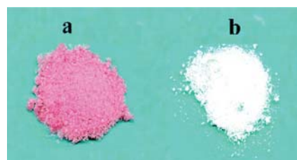
Fig. 2 Picture of poly(methyl methacrylate) (PMMA) synthesised by the RAFT process (a) before and (b) after reaction with AIBN. 45
