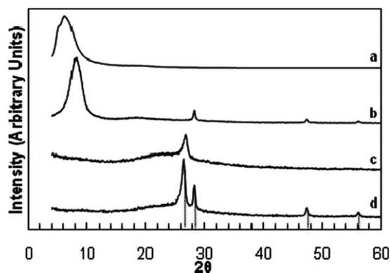
**Fig. 2** X-Ray diffraction patterns of: (a) GO paper; (b) SGO paper; (c) graphene paper by reduction of GO paper; (d) SG paper by reduction of SGO. Diffractions due to graphite ( $26.4^\circ$ ) and Si (111), (220), and (311) at  $28.3^\circ$ ,  $47.2^\circ$ , and  $56.1^\circ$ , respectively, are indicated.
