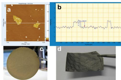
**Fig. 1** (a) and (b) AFM scan of two graphene oxide sheets, showing a single layer height of about 1 nm and about  $1 \times 1 \mu\text{m}$  wide (also determined by DLS, Fig. S3 (ESI<sup>†</sup>)). (c) Si-graphene oxide (SGO) composite paper. (d) Si-graphene (SG) composite paper obtained by reduction of SGO.
