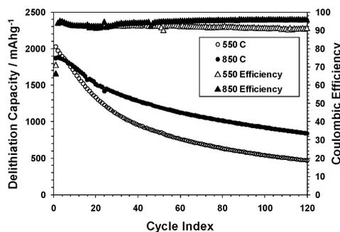
**Fig. 4** Delithiation capacities and coulomb efficiencies of SG samples reduced at 550 or  $850^\circ\text{C}$ , using a constant current–constant voltage (CCCV) method ( $1.5\text{--}0.020 \text{ V}$ ,  $1000\text{--}50 \text{ mA g}^{-1}$ ).
