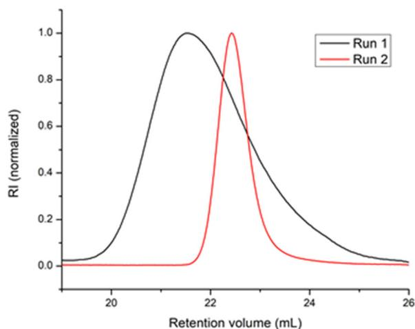
Fig. 1 SEC traces of polyethylene obtained with 1/BOMAG (run 1, Table 1) and 1/BOMAG/ZnEt<sub>2</sub> (run 2, Table 1) catalysts.
