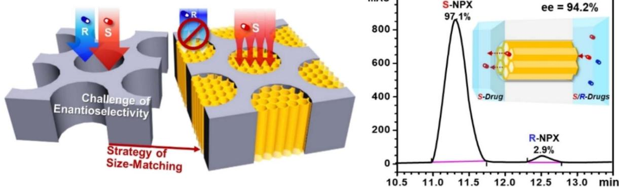
Fig. 29 Schematic representation of chiral COF-packed nanochannel membrane to solve the challenge of enantioselectivity and HPLC chromatogram of separated naproxen through the *L*-Tyr-COF channel membrane.<sup>76</sup> Reproduced with permission from ref. 76. Copyright 2022, John Wiley and Sons.
