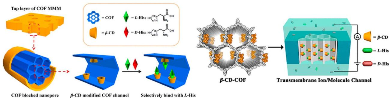
Fig. 28 Schematic representation of the construction of  $\beta$ -CD-COF MMMs and subsequent voltage-driven enantioselective transport.<sup>333</sup> Reproduced with permission from ref. 333. Copyright 2019, the American Chemical Society.
