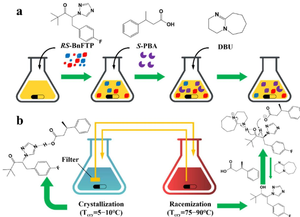
Fig. 13 (a) Schematic representation of the CoISD process and (b) the CoISD mechanism that occurred in a two-vessel setup with the cocrystal in suspension.<sup>55,239</sup> *RS*-BnFTP, PBA and DBU represent the racemic mixture, chiral coformer and racemizing agent, respectively.
