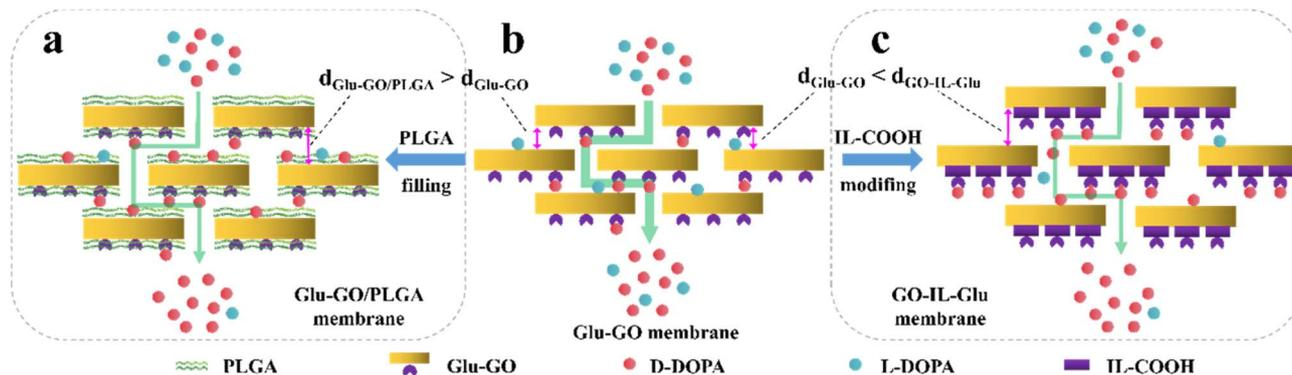
Fig. 25 Stylized illustration of (a) Glu-GO/PLGA, (b) Glu-GO and (c) GO-IL-Glu composite membranes.<sup>321,322</sup>
