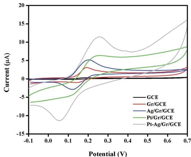
Fig. 5 Cyclic voltammograms of 25 μM DA in 0.1 mol L<sup>-1</sup> PBS (pH 6.5) at a scan rate of 20 mV s<sup>-1</sup> on bare GCE, Gr/GCE, Ag/Gr/GCE, Pt/Gr/GCE and Pt–Ag/Gr/GCE.
