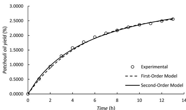
**Fig. 8** A comparison of the first-order and second-order kinetic models with the experimental results for the extraction of patchouli oil by the conventional method (hydrodistillation). The ratio of patchouli leaves to distilled water was 0.10 g mL<sup>-1</sup>.
