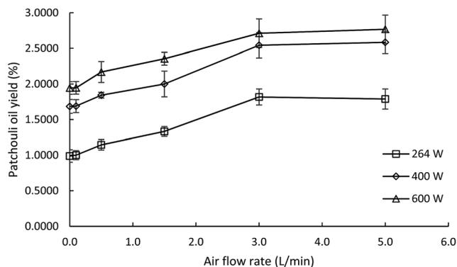
Fig. 3 The effect of the air flow rate on the yield of patchouli oil extracted at different microwave power levels. The ratio of patchouli leaves to distilled water was 0.10 g mL<sup>-1</sup>.
