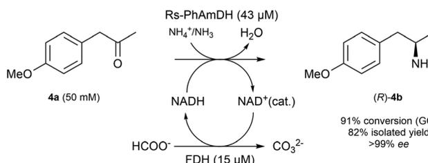
**Scheme 2** Preparative reductive amination of (*para*-methoxy phenyl)acetone (**4a**, 208 mg) using Rs-PhAmDH. Reaction conditions: ammonium formate buffer (1 M, pH 8.5), *T* 30 °C, agitation on an orbital shaker (190 rpm), reaction time 24 h.
