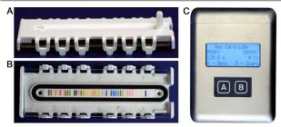
**Figure 1.** The optoelectronic nose. (A) The linear array of colorimetric sensors and disposable cartridge. Cartridge side view (7.9x2.8x1.0 cm). (B) Cartridge front view. (C) Handheld reader/analyzer (12.8x9.5x4.0 cm) based on a color contact line imager.
