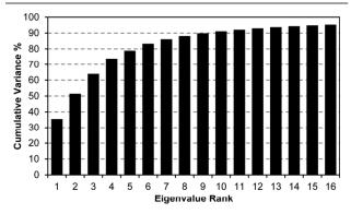
Figure 4. Scree plot of the principal component analysis for 15 explosives and related compounds. 16 dimensions were required to capture 95% of the total variance, consistent with the colorimetric sensor array probing a wide range of chemical reactivity.
