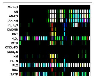
Figure 3. Difference maps of the 40-element colorimetric sensor array showing signal-to-noise of 16 explosives, related analytes, and the control. S/N ratios of 3-10 were scaled for display on an 8-bit RGB color scale (i.e., 0-255).
