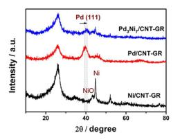
Fig. 3 XRD patterns of  $\rm Pd_3Ni_7/CNT\text{-}GR, Pd/CNT\text{-}GR,$  and Ni/CNT-GR.
