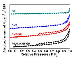
Fig. 1 N<sub>2</sub> sorption isotherms of CNT-GR and Pd<sub>3</sub>Ni<sub>7</sub>/CNT-GR.
