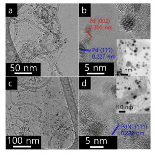
Fig. 2 TEM images of Pd/CNT-GR (a,b) and Pd<sub>3</sub>Ni<sub>7</sub>/CNT-GR (c,d).
