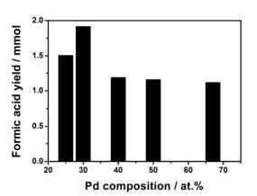
Fig. 5 Formic acid yields as a function of Pd content. Reaction conditions: 1 mmol (Pd+Ni) catalysts, 90 ml H<sub>2</sub>O, P = 50 bar (H<sub>2</sub>/CO<sub>2</sub> = 1), 40  $^{\circ}$ C, 15 h.
