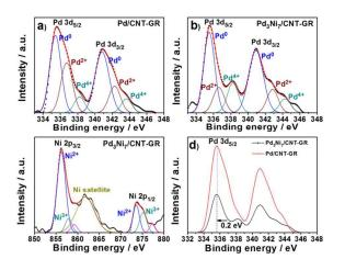
Fig. 4 Pd 3d and Ni 2p XPS spectra; a) Pd in Pd/CNT-GR, b) Pd in Pd<sub>3</sub>Ni<sub>7</sub>/CNT-GR, c) Ni in Pd<sub>3</sub>Ni<sub>7</sub>/CNT-GR, and d) comparison of Pd spectra in Pd/CNT-GR and Pd<sub>3</sub>Ni<sub>7</sub>/CNT-GR.
